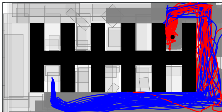
Figure 4.20: Red curves indicate the routes followed by the robot and darker nodes represent the newly generated nodes after resampling procedure.
