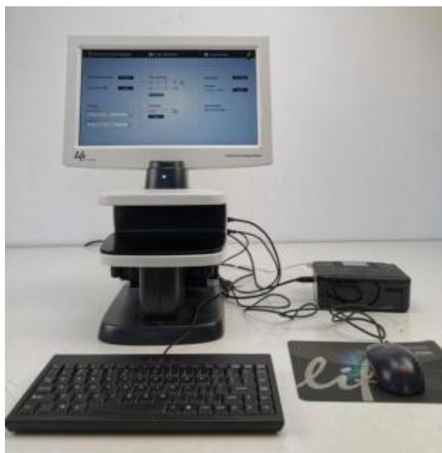
Figure 2.1 EVOS Fluid Cell Imaging Station used to visualize B.subtilis spores
