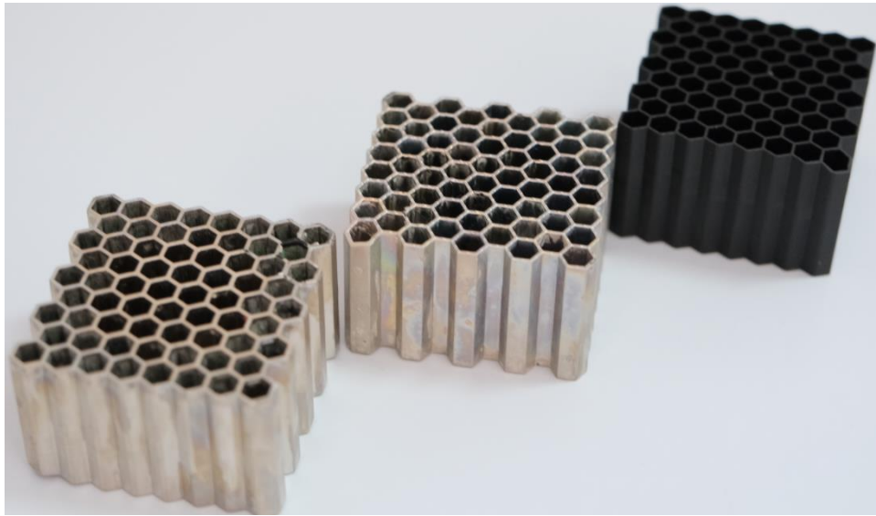
Figure 4.1. Image of a virgin uncoated RPU 70 honeycomb lattice structure next to post-mortem electroplated samples.
