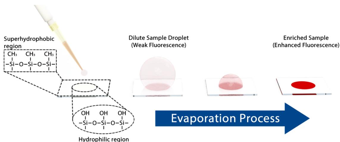
**Figure 1.** Schematic representation of droplet pinning on superhydrophilic circular pattern of a superhydrophobic ormosil surface and evaporation-induced enrichment of low-concentration, low-volume fluorescent sample and resulting fluorescence enhancement.
