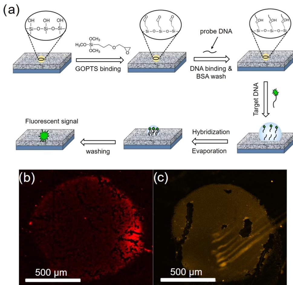
**Figure 5.** (a) Schematic representation of epoxysilane binding onto UV/ozone-treated regions, followed by attachment of probe DNA, hybridization of fluorescence-tagged target DNA, evaporation-induced analyte enrichment, and fluorescence enhancement. (b) Confocal image of wetted pattern after the attachment of Cy5-tagged probe DNA. (c) Confocal image of wetted pattern after hybridization of probe DNA with 20 pM Cy3-tagged target DNA in 4  $\mu\text{L}$  of evaporating droplet.
