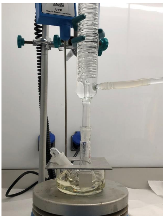
Figure 2.4. Photograph of the batch experimental setup used for PLA degradation
