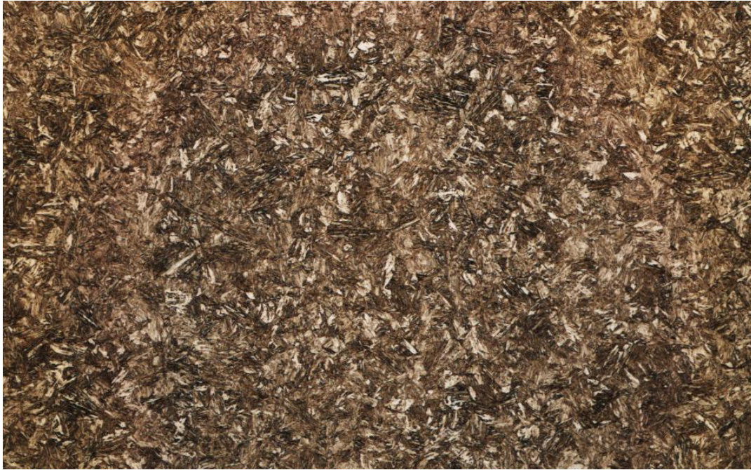
Figure 4.3. A representative microstructure after pre-hardening, 200x
