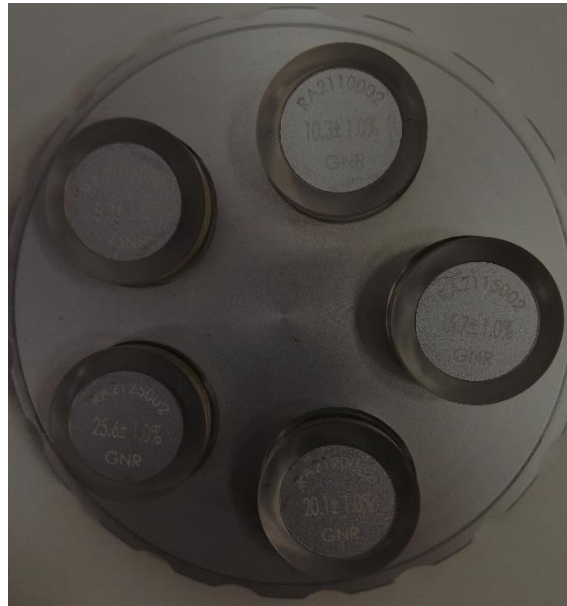
Figure 4.4. Retained austenite calibration blocks
