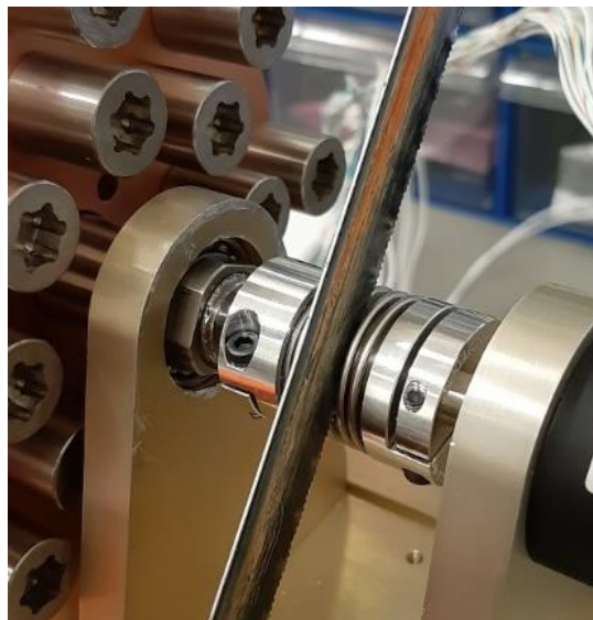
Figure 5.12. Cutting of a single bellow section on the metal bellow coupling
