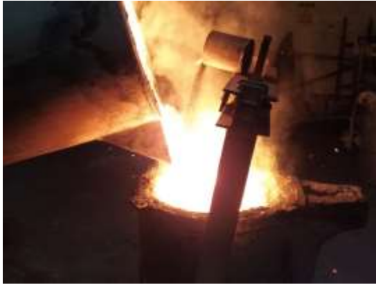
Figure2. 3: Ladle inoculation before pouring the melt.
