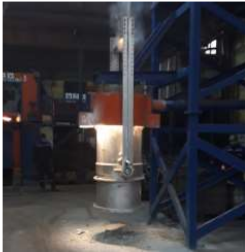
Figure2. 2: Cored wire Mg treatment for nodular graphite cast iron.
