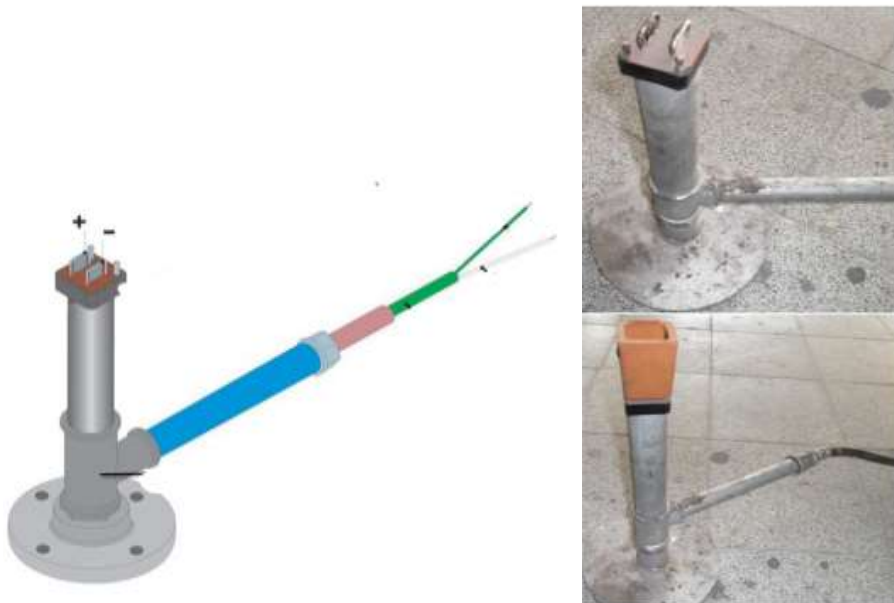
Figure2. 6: Quick up test sample port for thermal analysis.
