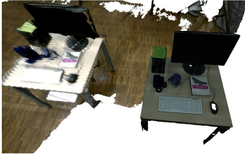
Figure 5.9: Dense 3D model of the scene obtained by our proposed methodology (Close up view)
