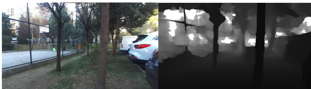
Figure 3.2: Output images of RGB-D sensors. Left: RGB image. Right: Depth image. The brighter a pixel is, the farther away it is from the sensor.
