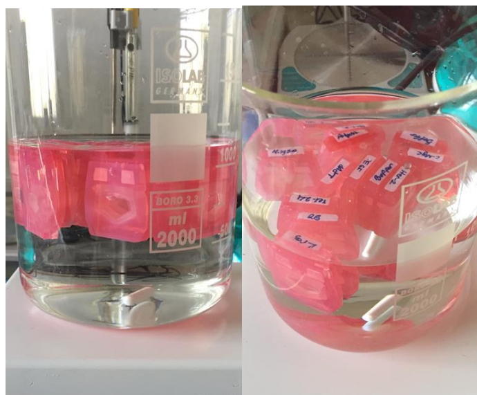
Figure 2.1. Competition Dialysis set-up. Disposable dialysis cassette, each containing 600.0 \mu\text{L} of a 75.0 \mu\text{M} solution of one of the DNA structures listed in Table 2.3, are placed in a beaker containing 750.0 mL of 1.0 \mu\text{M} ligand solution in 1XBPES.
