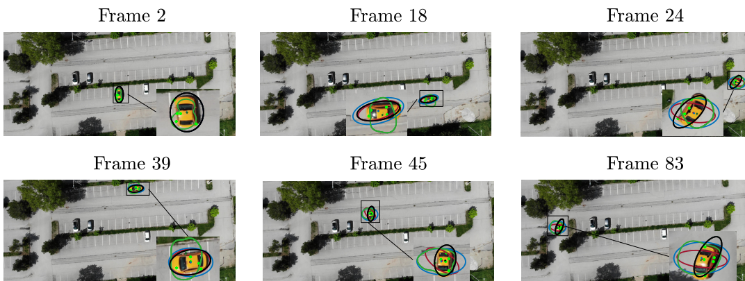
Figure 3.5: A representative MC run of the real data experiment. The extent estimates of VB, Algorithm-1, Algorithm-2, and GP-ETT are shown in black, red, blue, and green lines, respectively. The measurements are represented with green dots.
