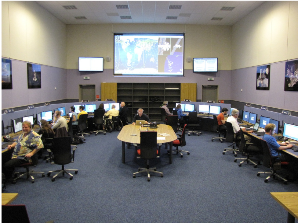
Figure 3.3: AMS POCC at CERN close to Geneva. In the middle screen the orbit of ISS is being followed live. Shift takers and experts in different desks watch different systems such as thermal system, data acquisition and the operation of specific sub-detectors [37]
