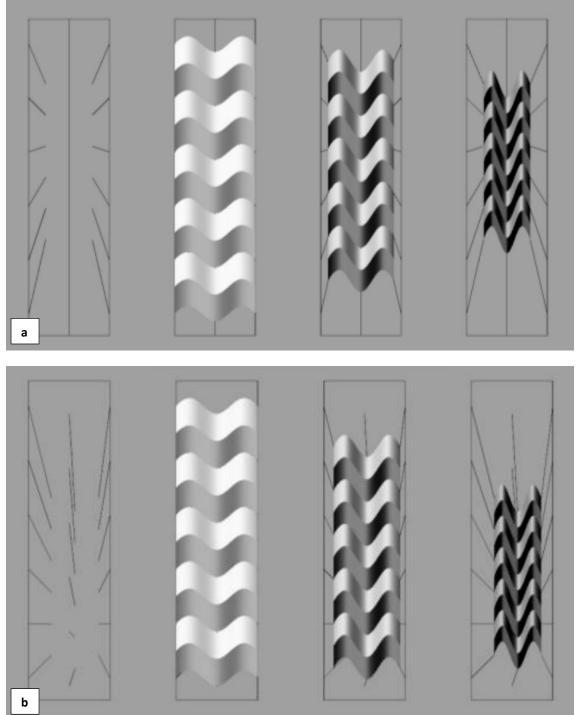
Figure 5: Generation of the grid based on applied forces and the symmetry group. Surfaces in Figure 5a and 5b have the same modules yet with distinct directions of the applied forces (developed by the authors)
