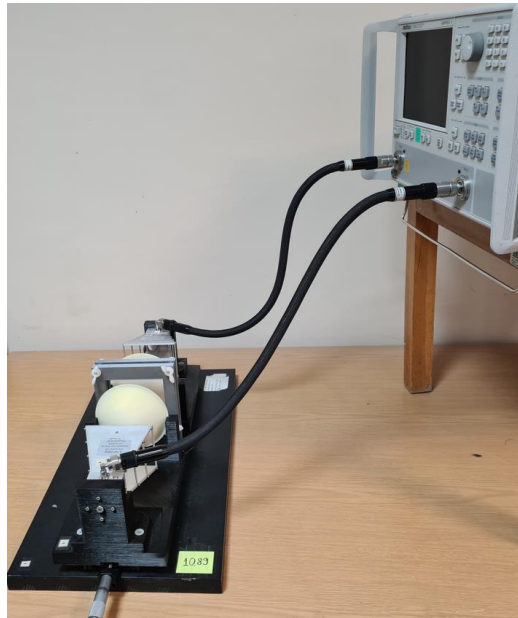
Figure 3.1. Measurement setup for dielectric characterization.
