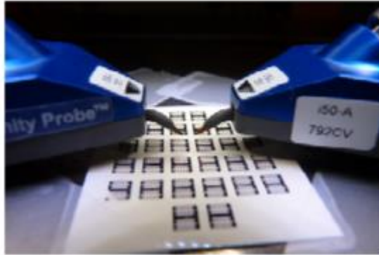
Figure 2.7. Measurement method of BST IDC [43].
