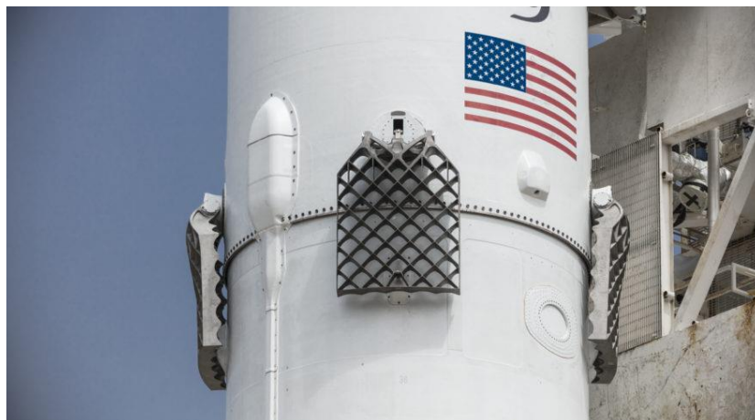
Figure 1.5. SpaceX Falcon9 Reusable Launch Vehicle Equipped with Grid Fins [5]
