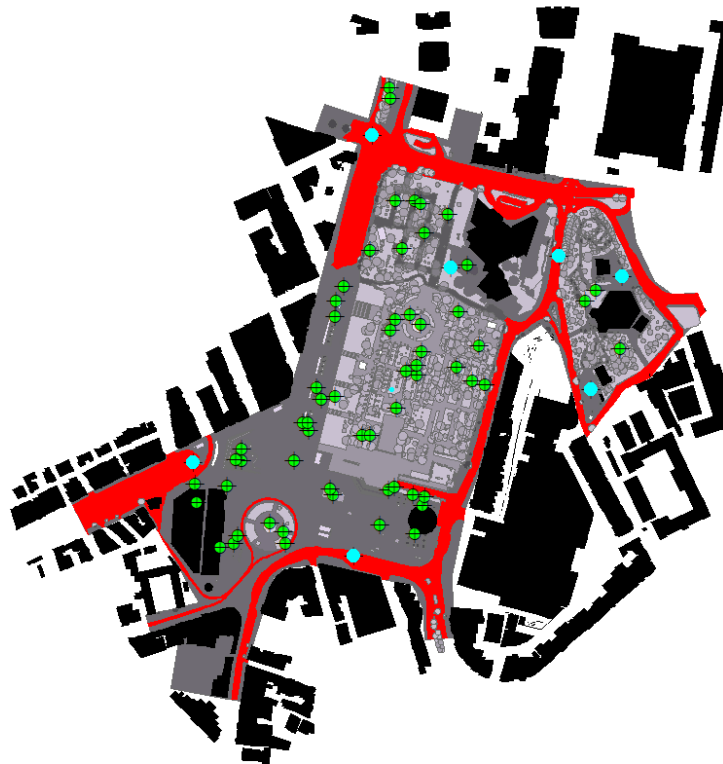
Figure 3.12 The surface temperature measurement points (cyan points) on asphalt surfaces (red surfaces)
