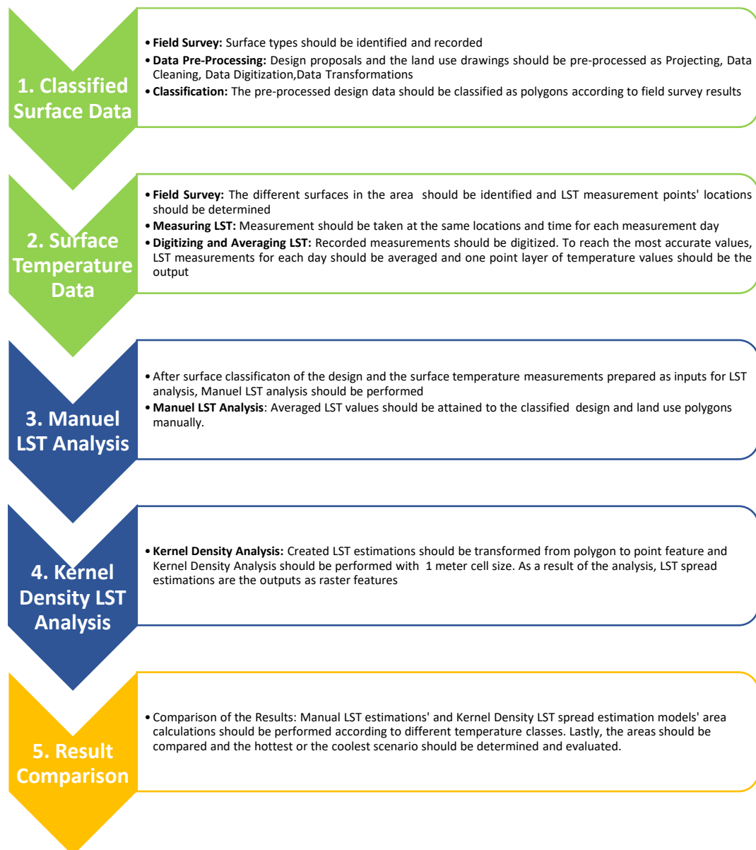
Figure 3.20 Procedure to implement LST Estimation Model in an urban design process
