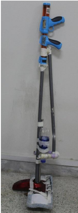
Figure 5.18: The stand can be seen latching on to the bottle, it also opens up to become a support for the structure so to not have to lean against a wall.
