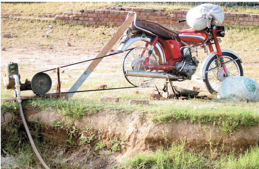
Figure 2.10: A motorbike being used as an extension for a water pump
