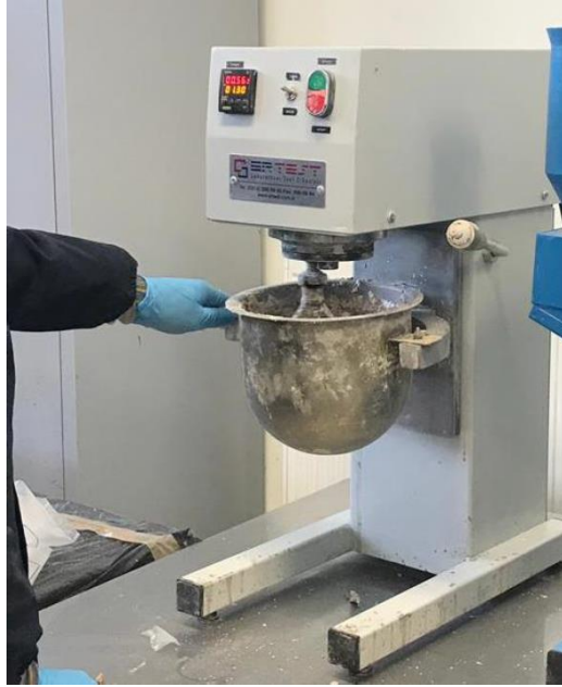
Figure 3-14: Mixing raw materials with mixer
