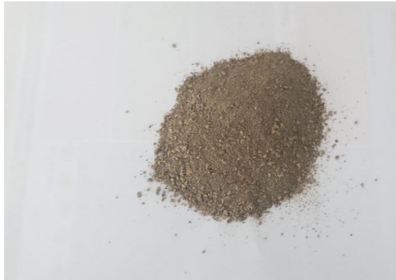
Figure 3-12: Jacaranda Seed Pod Pulverized
