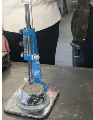
Figure 4-6: Vicat Apparatus and mold with sample
