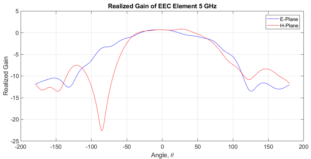
Figure 4.8: EEC Element simulation gain pattern at 5 GHz.
