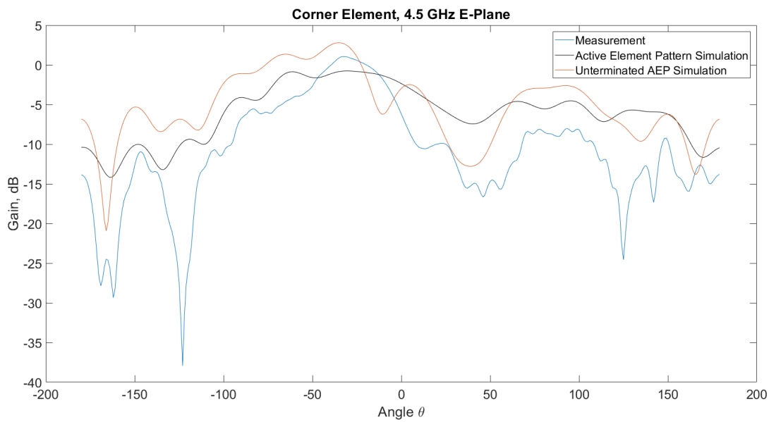
Figure 4.25: Corner Element E-plane gain pattern at 4.5 GHz, Measurement and simulation comparison.
