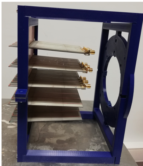
Figure 4.18: Fabricated 5×5 TCDA array, side view.
