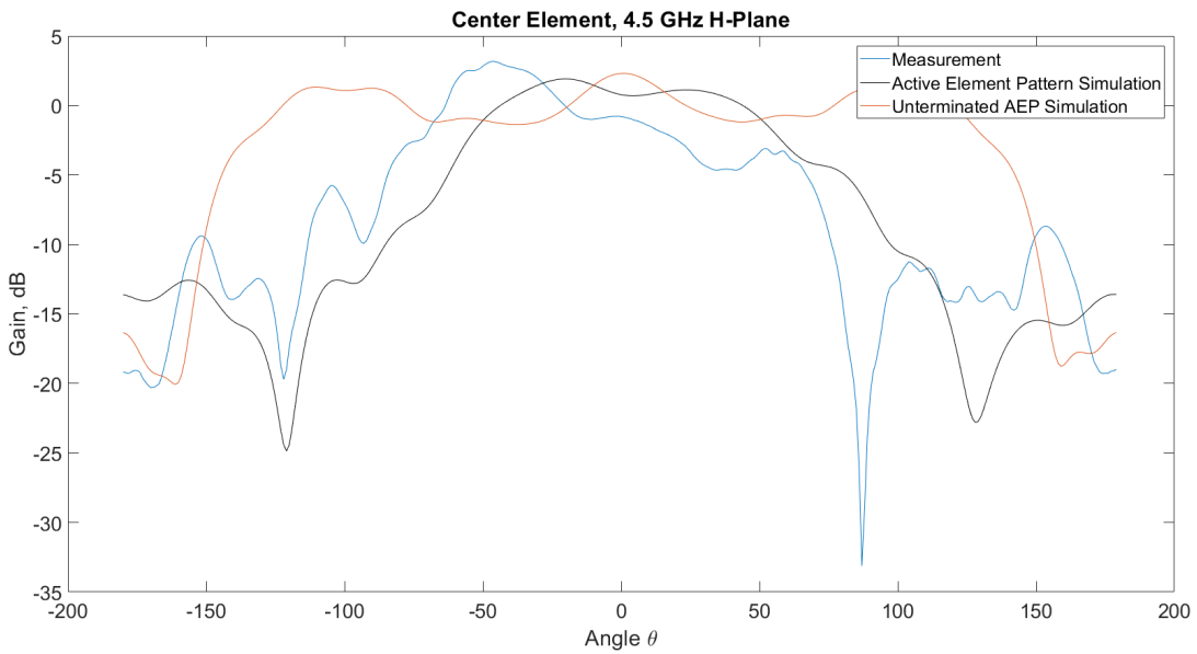
Figure 4.30: Center Element H-plane gain pattern at 4.5 GHz, Measurement and simulation comparison.
