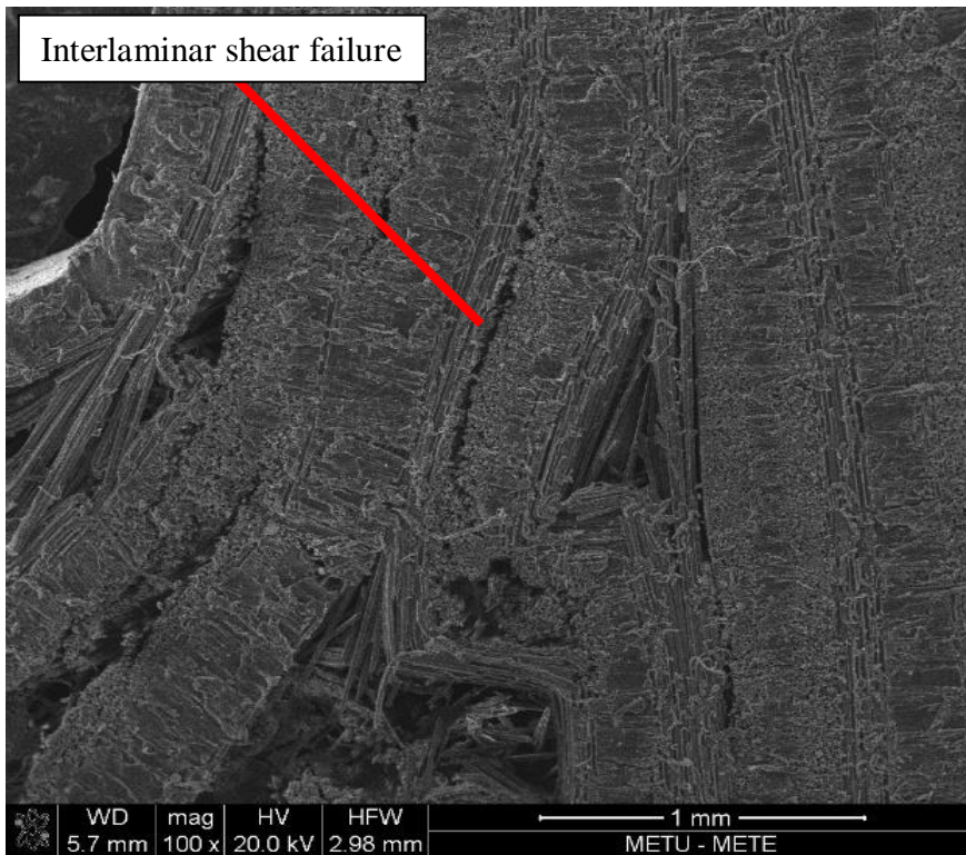
Figure 3.11. Through-thickness SEM images showing certain interlaminar shear failure in the PLA/GF laminate specimens
