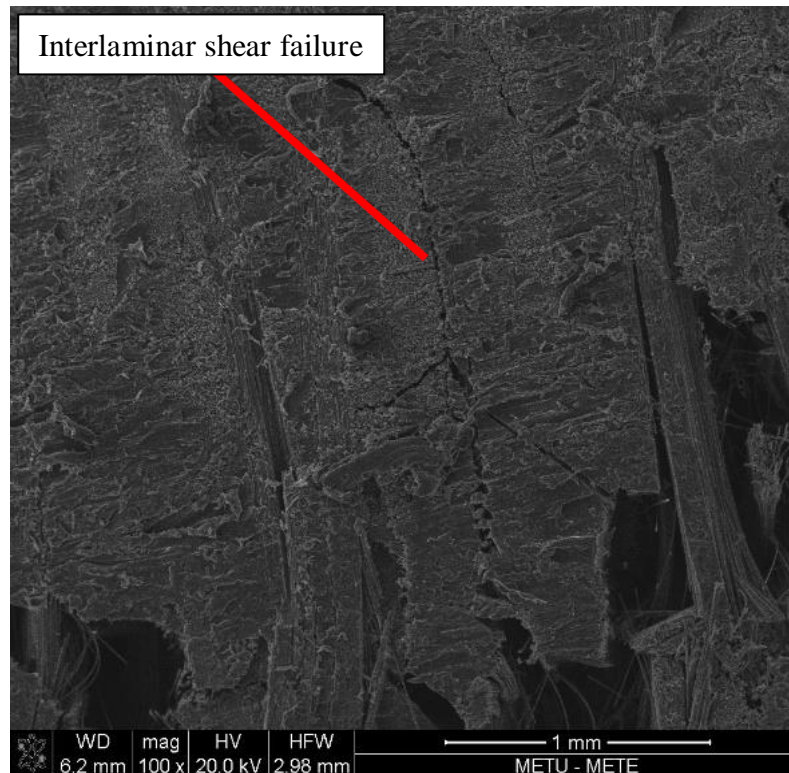
Figure 3.12. Through-thickness SEM images showing certain interlaminar shear failure in the PLA/CF laminate specimens
