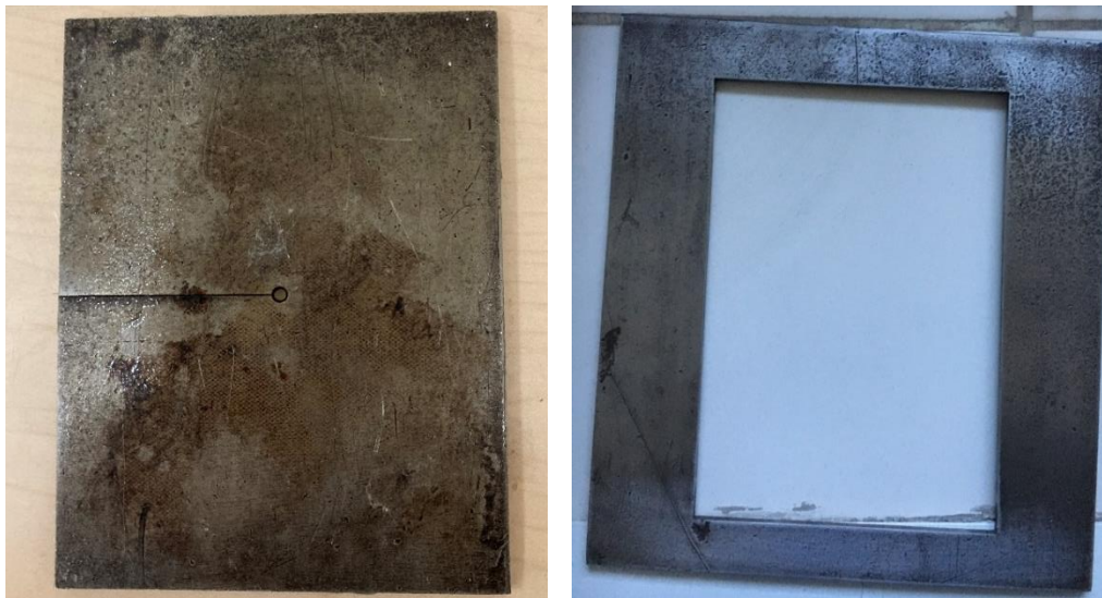
Figure 2.7. Pieces of the mold machined from a steel plate
