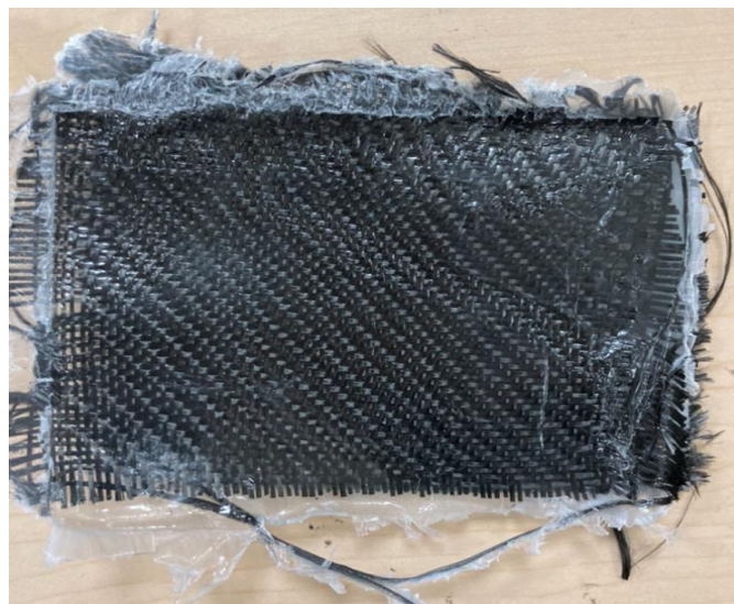
Figure 2.13. An example of the PLA/CF composite laminate plate produced
