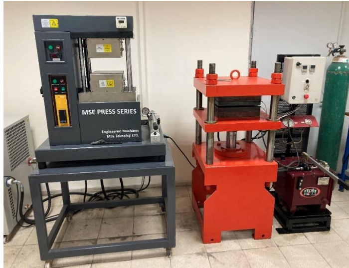
Figure 2.12. Hot press (left) and cold press (right) used for the consolidation by compression molding
