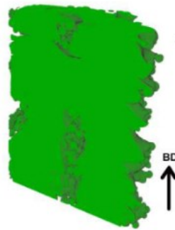
Figure 3.7. Section cut of a 1.5 mm strut produced with “Net” theme [62].
