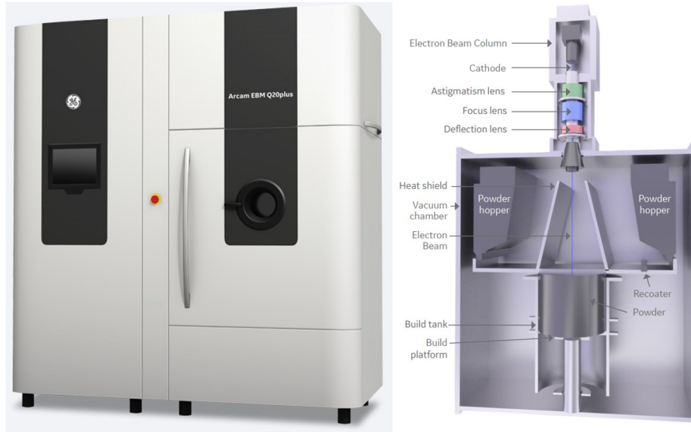
Figure 3.1. Arcam EBM Q20plus machine on the left and the layout of EBM system is on the right [52].
