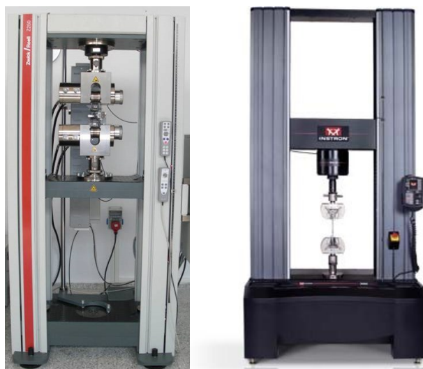
Figure 3.17. Machines used in experimental study (Zwick Z250 and Instron 5985).
