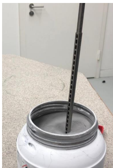
Figure 3.8. Sampling of powders by using designed apparatus
