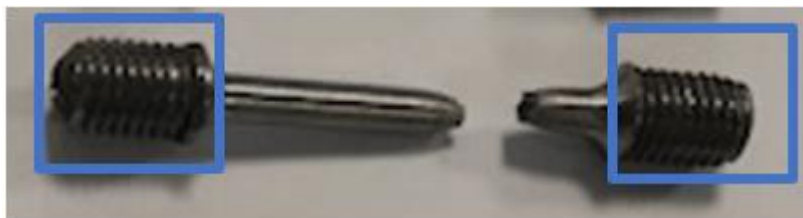
Figure 3.10. The ends of the tensile test specimen
