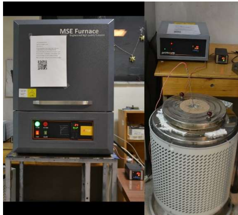
Figure 3.1. Heat treatment equipment used for experiments: MSE Furnace M1200 open atmosphere muffle furnace (left), PROTHERM Furnaces PCF 10/250/400 salt bath furnace (right)
