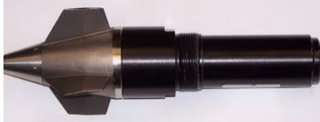
Figure 1.4: An Example Design Which Uses Fixed Aerodynamic Surfaces
