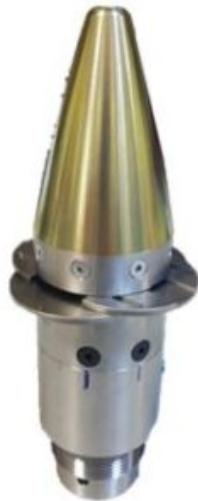
Figure 1.1: An Example Design of 1-D Control Approach by Using Drag Brake
