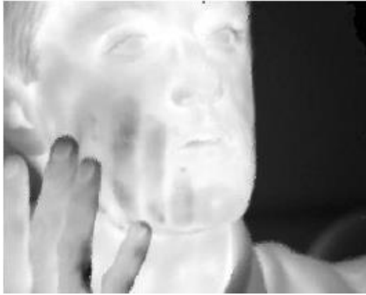
Figure 2.13: Thermal image taken by 320 \times 256 InAs/GaSb nBn based superlattice with 16.3 ms integration time at 77 K [80].
