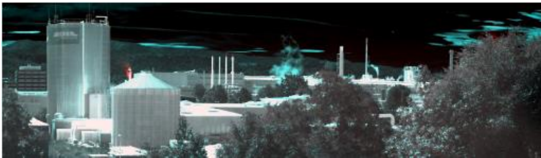
Figure 2.14: The infrared image taken with 384 \times 288 dual-color InAs/GaSb SL camera. The blue channel corresponds to between 3\text{-}4 \mu\text{m} and the red channel corresponds to between 4\text{-}5 \mu\text{m} are represented by cyan and red colors, respectively [81].
