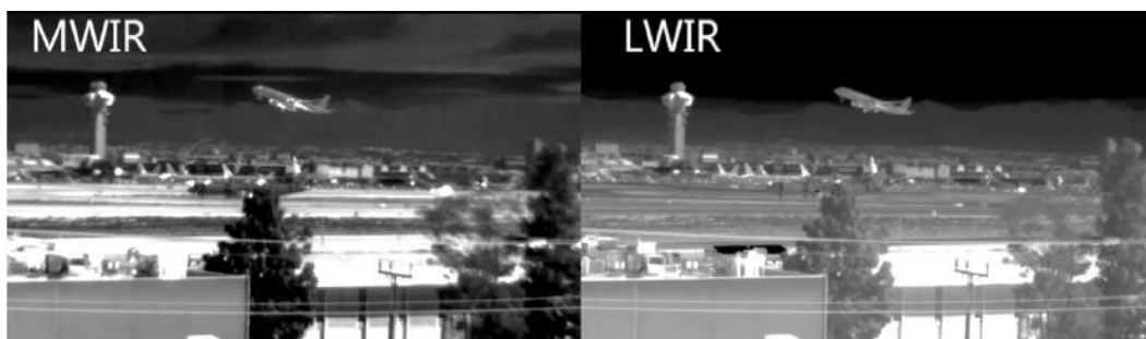
Figure 1.4: Images taken by dual-band MW/LW SLS FPA fabricated on VISTA at 80 K [15].
