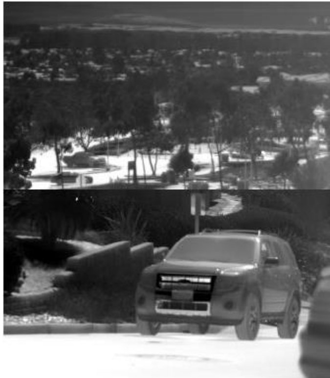
Figure 2.23: Images captured with 5 \mu\text{m} pitch 1k \times 2k array size MWIR FPA at 150 K [92].
