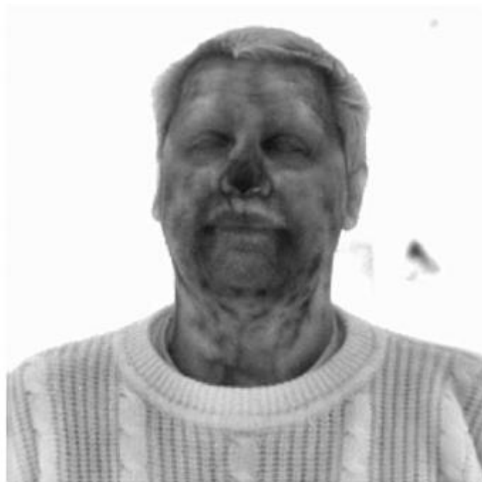
Figure 2.10: The image was taken by the first superlattice 256 \times 256 MWIR FPA by Walther et al. in 2005 [48].
