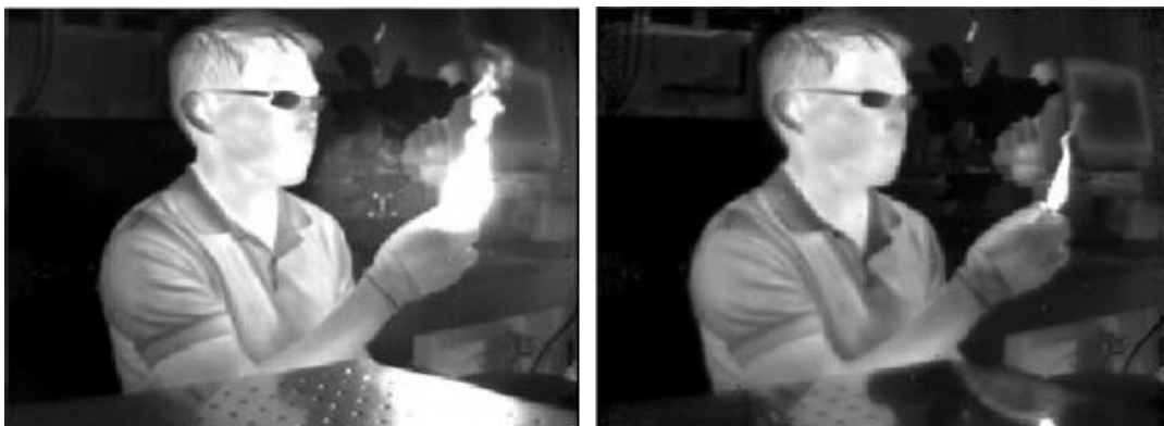
Figure 2.16: Thermal image taken with dual-band 256 \times 320 T2SL FPA [84].
