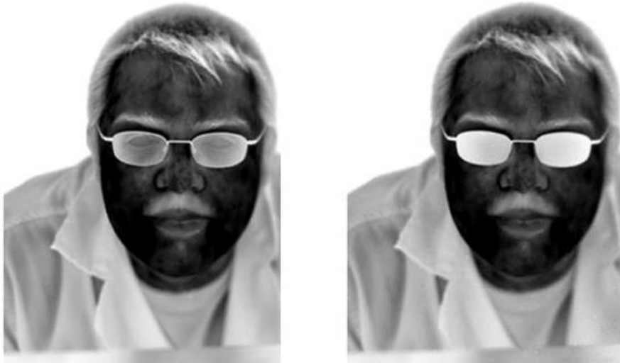
Figure 2.15: Thermal images taken with dual-color FPA. The left is the blue channel, and the right is the red channel [83]. White regions correspond to the colder places.
