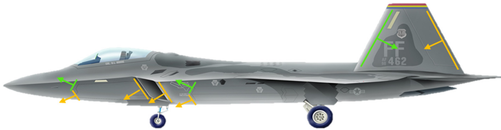
Figure 1.9 Angular alignment on representative geometry of F-22 Raptor aircraft from the side view
