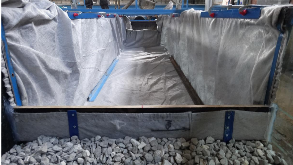
Figure 3.5 Placement of the Geotextile Filter
