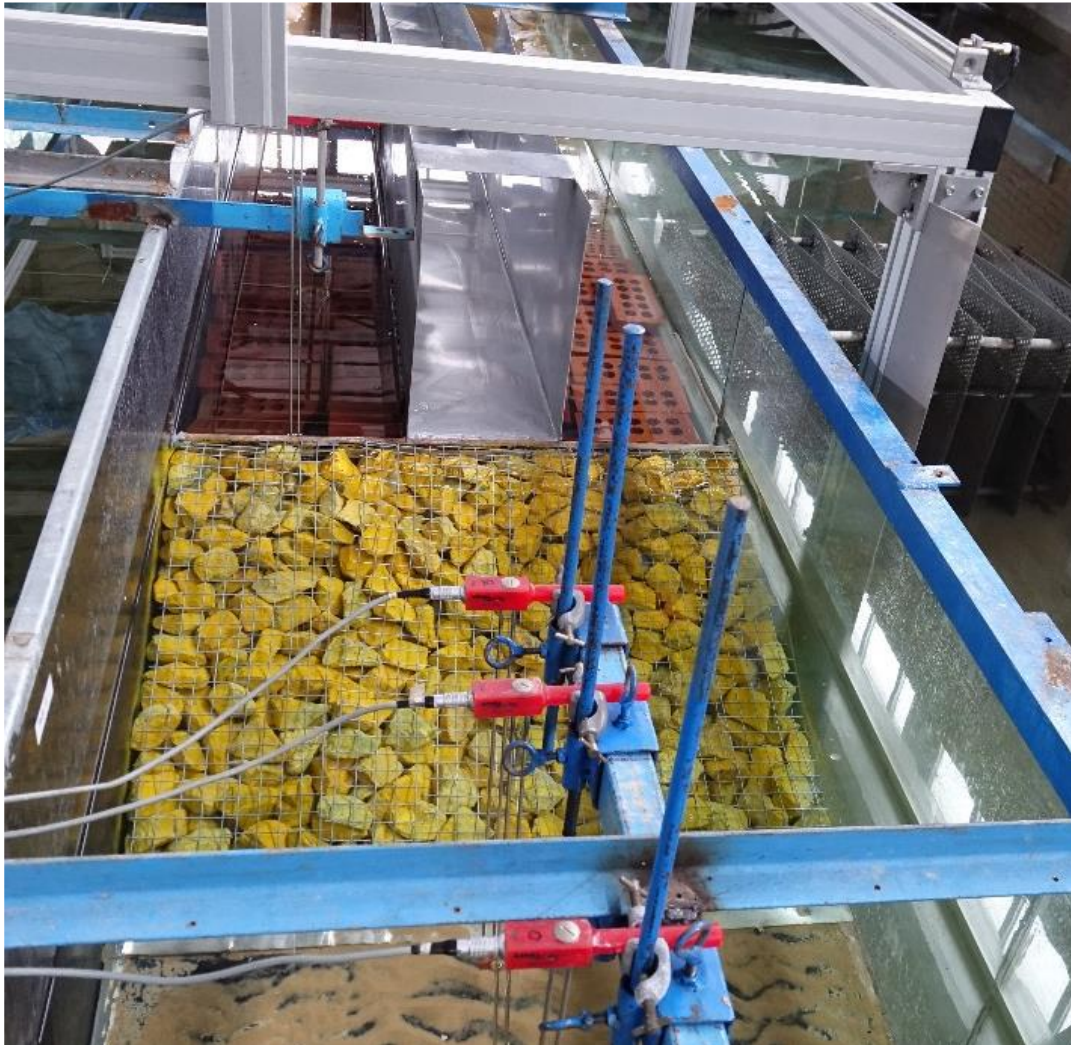
Figure 3.10 Overtopping Gutter on the Revetment
