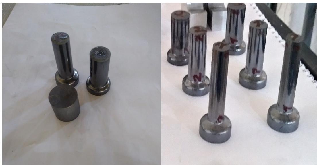
Figure 1. (a) an initial material and cold extruded specimens (b) the cold extruded specimens at three true strain
