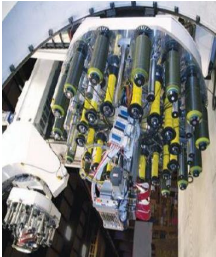
Figure 2.12 AFP machine head with multiple tows
