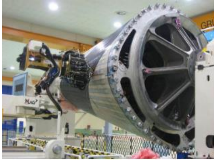
Figure 2.21 AFP manufacturing of the fuselage section of Airbus A350
