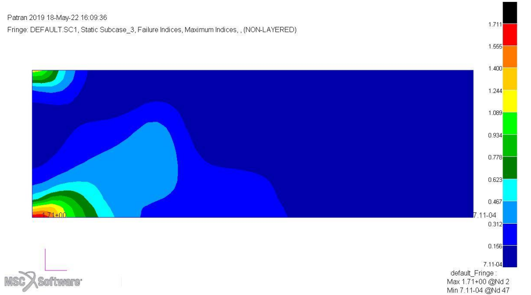
Figure 6.25 FI plot of the flat panel with the initial reference path under the given load and boundary conditions
