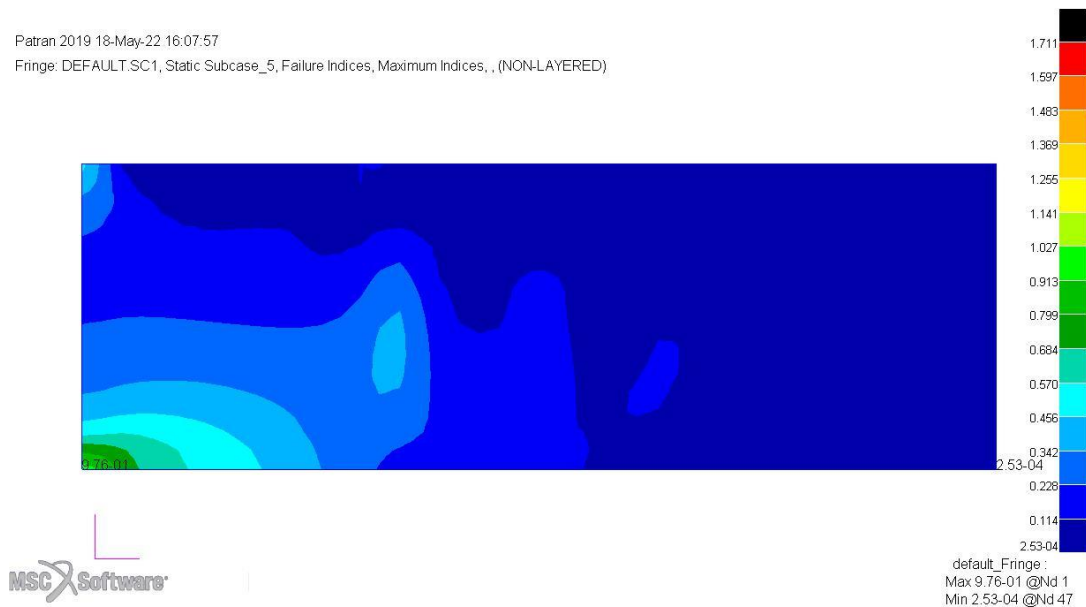
Figure 6.26 FI plot of the flat panel with the optimized fiber path under the given load and boundary conditions
