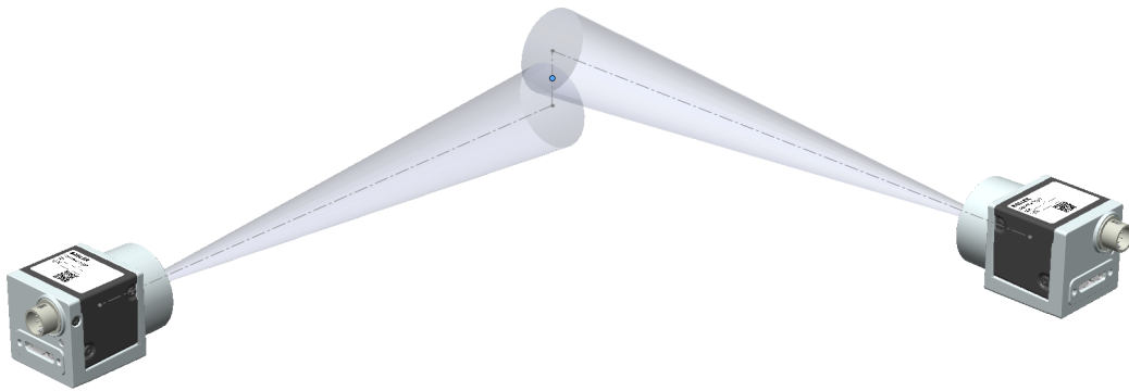
Figure 3.2: Position Estimation from Camera Measurements
