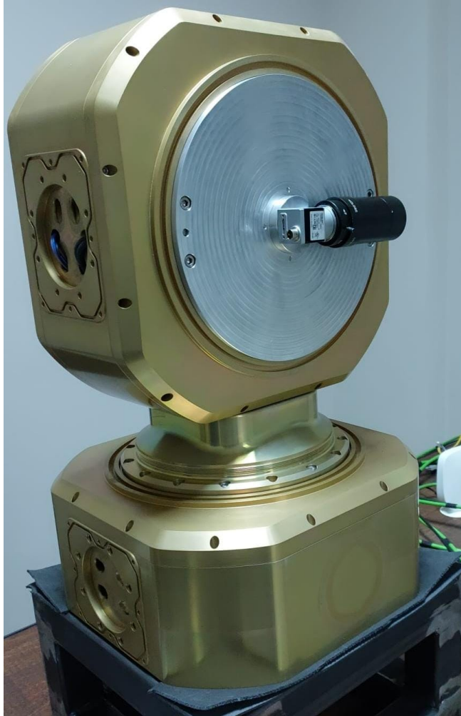
Figure 4.1: Gimbal with Camera
