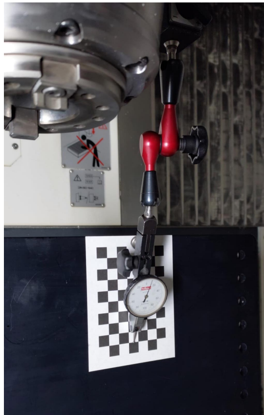
Figure 4.8: The Dial Gauge with Calibration Pattern
