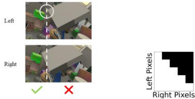
Figure 3.8 (a) Geometric constraints of stereo matching, (b) the attention mask [61]
