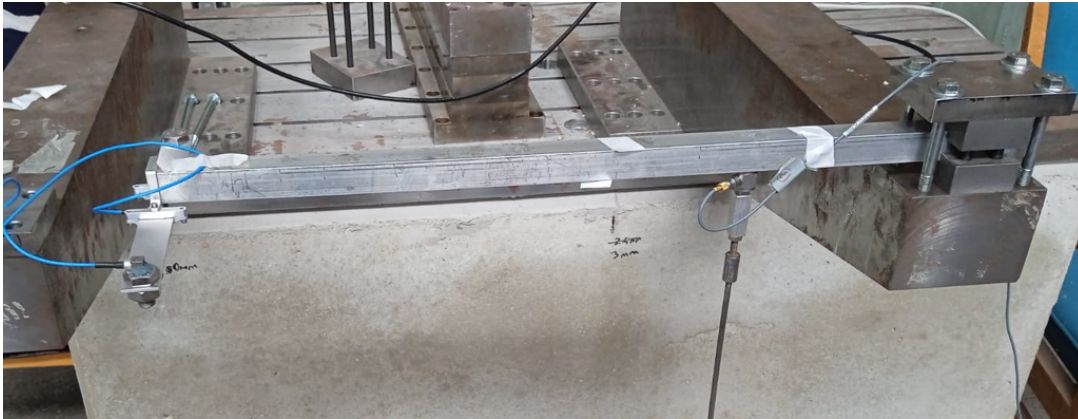
Figure 5.11: Test Setup for TVA Transmissibility Measurement
