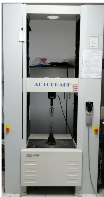
Figure 3.13 Shimadzu Autograph AG-IS 100kN universal testing machine.
