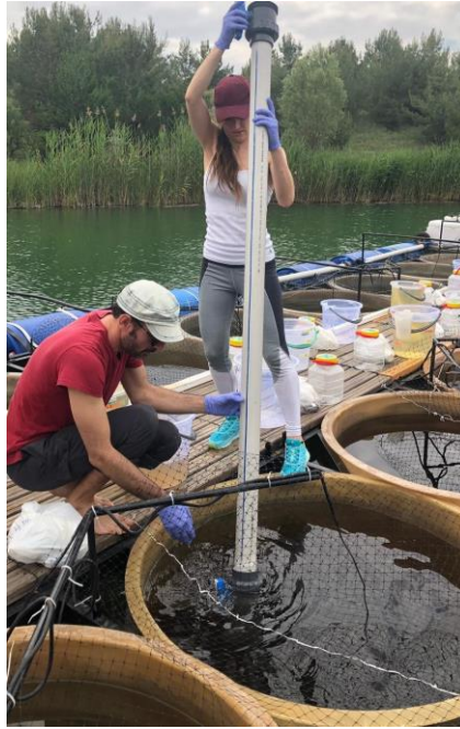
Figure 2.6 Surface to bottom tube sampling process to obtain depth-integrated mixed mesocosm water from each tank.
