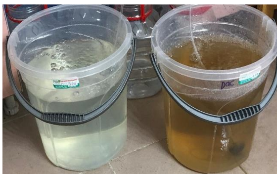
Figure 2.2 The - DOC (left) and + DOC (right) buckets at the beginning of the experimental setup.
