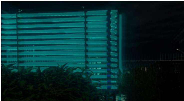
Figure 2.19. Bioluminescent bioreactor developed by the company that can control the bacteria and necessary nutrients in the system, refill and clear it (Glowee, 2016).
