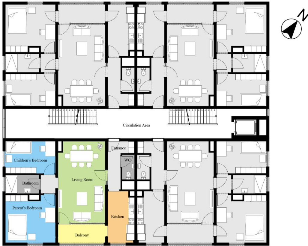
Figure 3.2. Architectural plan of a typical floor of the 14th block building consisting of four flats and the selected flat on the 13 th floor with color coding where the lighting measurements and simulations were done.
