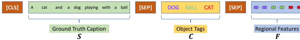
Figure 4.3: Input sequence to transformer for VinVL [4] for the example provided in Figure 4.1.
