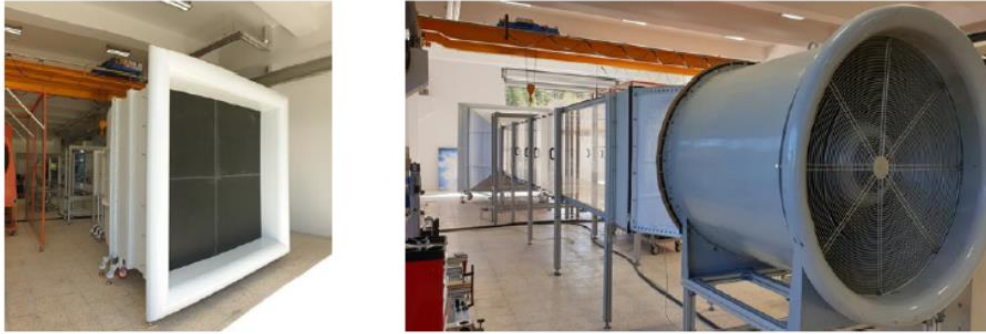
Figure 2.1: RÜZGEM C3 open-loop suction type wind tunnel
