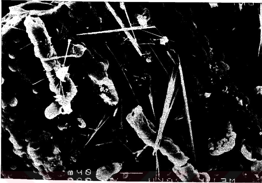
Figure 3.30.: Scanning electron micrograph showing fibrous zeolites (Erionite ? or mordenite ?) on silicified wood, X 1000, Sample No: BK-7.
