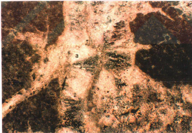
Figure 3.8.: Photomicrograph showing the aragonite cement of cherty limestone facies, (a) Aragonite, (Sample No: YT-25-01, Mag. X45, XPL)
