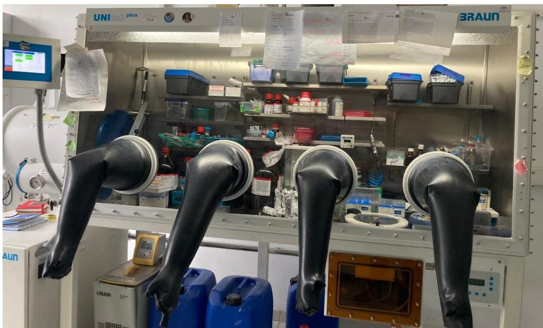
Figure 3.2. Nitrogen filled glove box to create an oxygen free environment for the processing of oxygen-sensitive materials.
