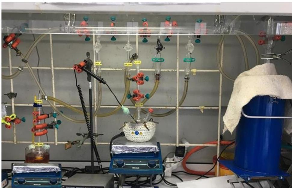
Figure 3.1. Schlenk line for the synthesis of air sensitive PbSe QDs and NRs.
