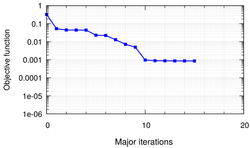
Figure 3.31: The evolution of the objective function with major optimization steps for case III
