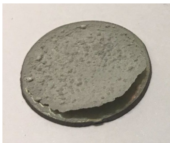
Figure 2.3 Image of A/G/20BHT after adhesion strength test.
