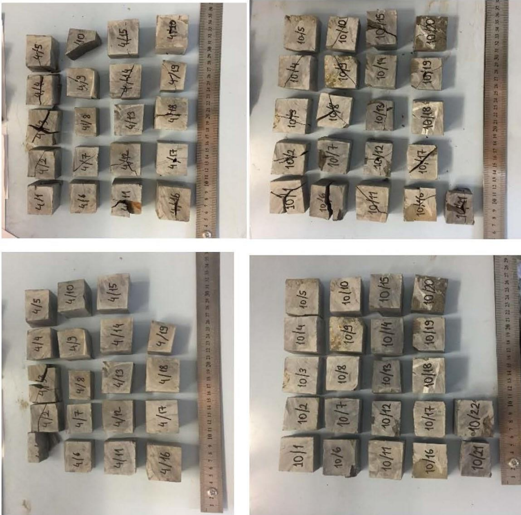
Figure C 1: The block samples of Sector 4 and Sector 10 before and after the Point Load Strength Index testing
