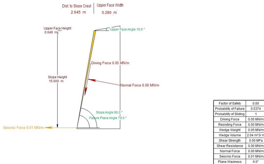
Figure 74: 2D view of the block generated for the pseudo-static analysis in Sector 8 by Rocplane software
