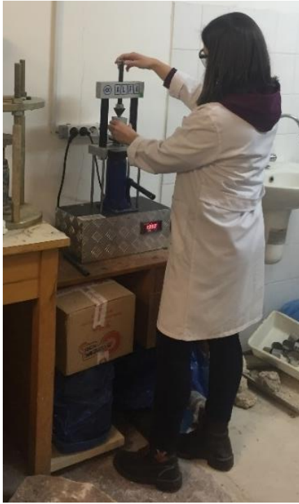
Figure 20: A view of Point Load Strength testing
