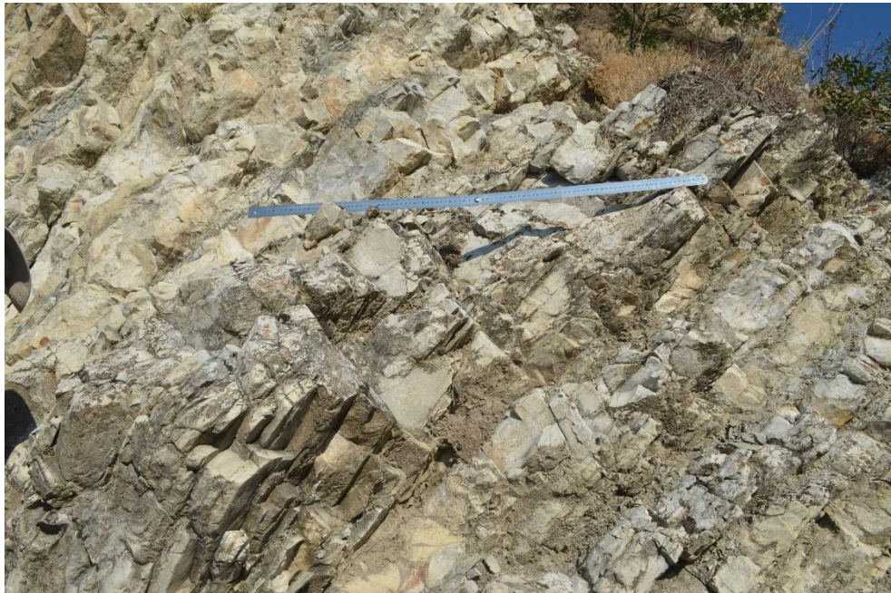
Figure 17: A close-up view of discontinuous limestone. Note the 2 m long measuring tape as a scale
