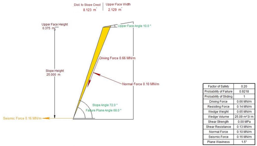
Figure 71: 2D view of the block generated for the pseudo-static analysis in Sector 4 by Rocplane software
