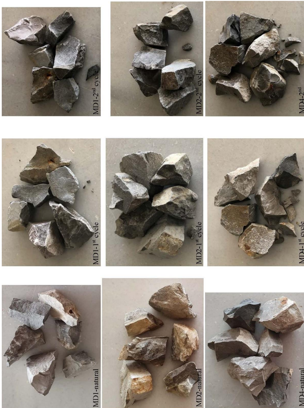
Figure C 2: Slake Durability tested rock samples from Sectors 1, 2 and 4. The first column shows a view of specimens before the test, whereas the second and third columns present the condition of the specimen following the 1 st and 2 nd cycles, respectively
