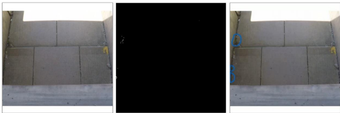
Figure 3.13: No movement state. Left to right; recorded frame, background subtraction mask output, and contours created by mask output
