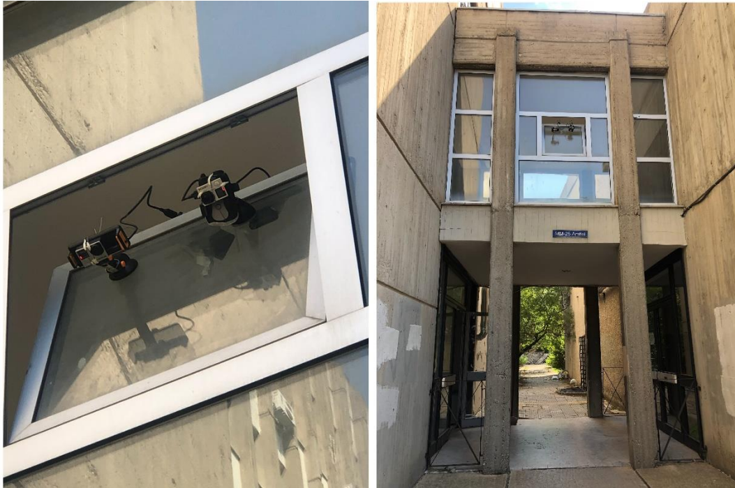
Figure 3.7: Camera attachment using suction phone mounts
