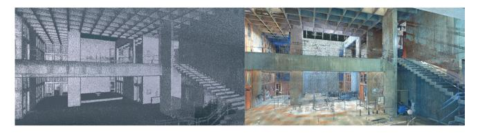
**Figure 7.** Point cloud model scanned with a low precision scanner (left), and with a high precision scanner (right) (Model made by Şahin Akın).
