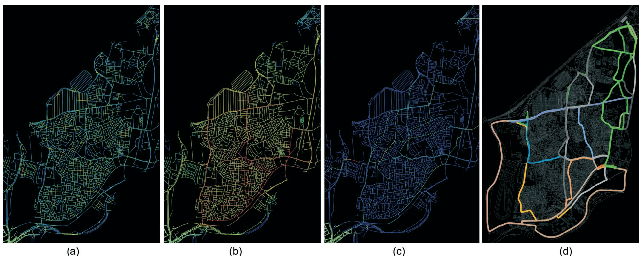
Figure 4. Space Syntax analysis of Zeytinburnu District from DepthMapX (a) Connectivity, (b) Integration, (c) Metric Choice Analysis and (d) Generated routes
