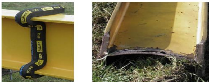
Figure 2-10 Bendability and Functioning of Chemring FLSC [15]
