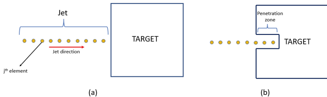
Figure 4-6 Sketches of Jet Element Movement (a) and Penetration to Target (b)
