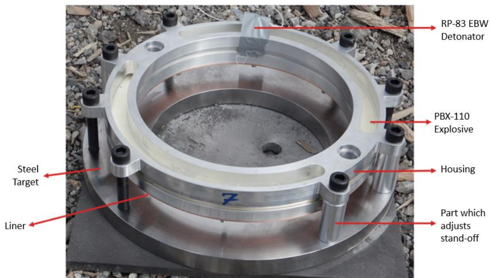
Figure 3-12 CLSC (On Plane) Test Set-up
