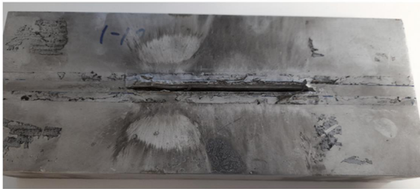
Figure 3-10 LSC, Target Top View after the Penetration
