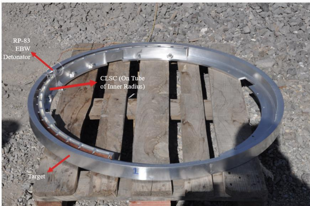
Figure 3-17 CLSC (On Tube of Inner Radius) Test Set-up
