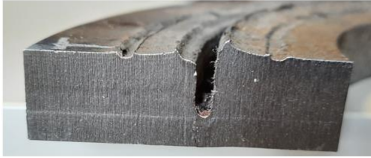
Figure 3-15 CLSC (On Plane) Penetration on Target (Cross-sectional View)
