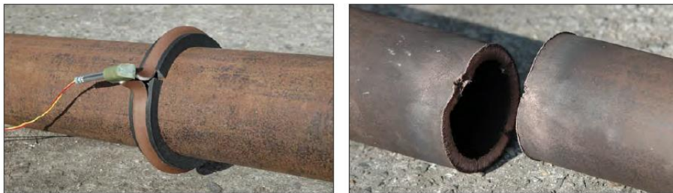
Figure 2-9 Bendability and Functioning of Explosia FLSC [14]
