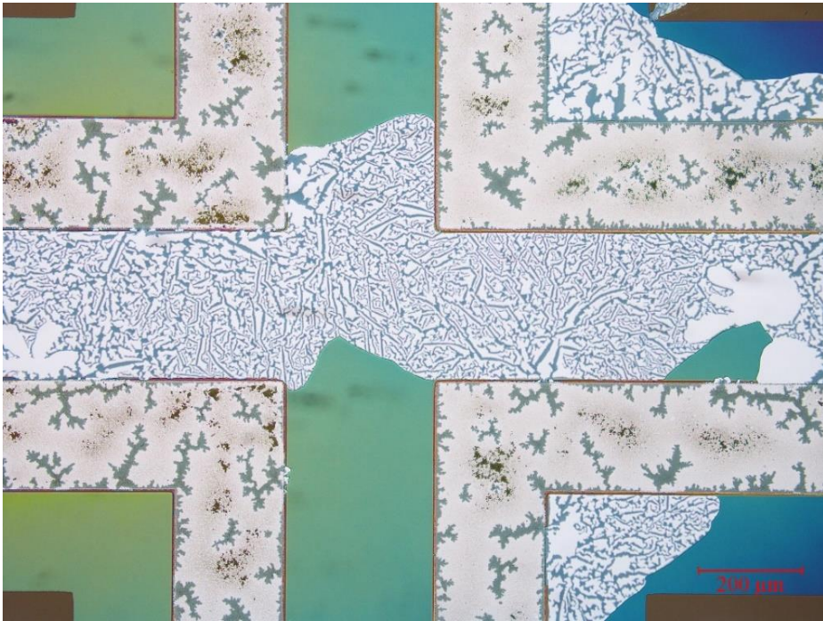
Figure 4.46 OM image of the wafers through the glass wafer after bonding at 435°C
