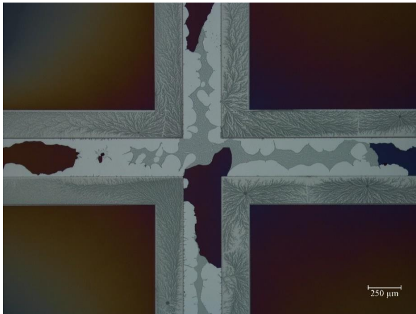
Figure 4.35 OM image of the bonding area through the glass wafer
