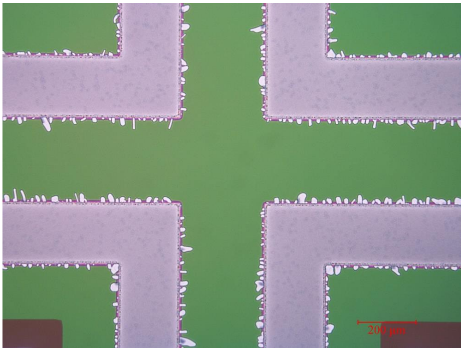
Figure 4.47 OM image of the wafers through the glass wafer after bonding at 430°C
