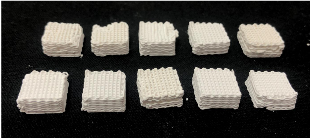
Figure 5.7: 3D Printed TCP Scaffolds with the optimized parameters: LPR:0.6, Binder Concentration: 25 wt.%, Tip I.D:0.4 mm, Printing Speed:9 mm/s
