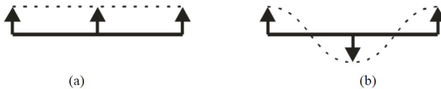
**Figure 1.6.** Rigid-body motion (a) and elastic deformation (b) on the surface of an optical component under random vibration [3].
