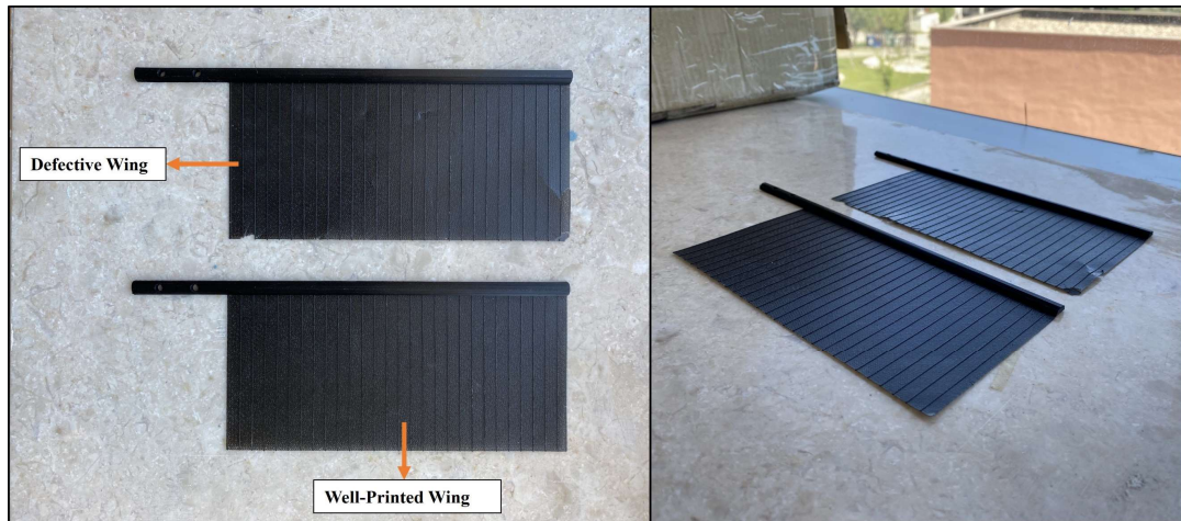
Figure 3.8. Defective wing and well-printed wing
