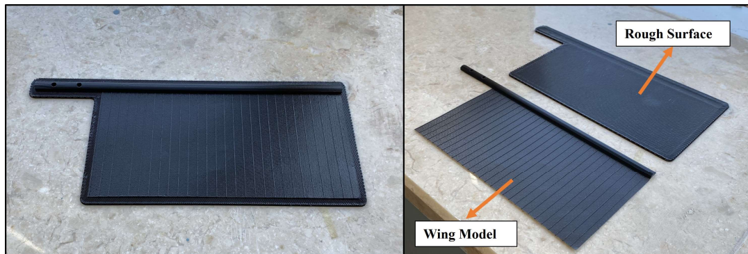
Figure 3.5. Rough surface and wing model
